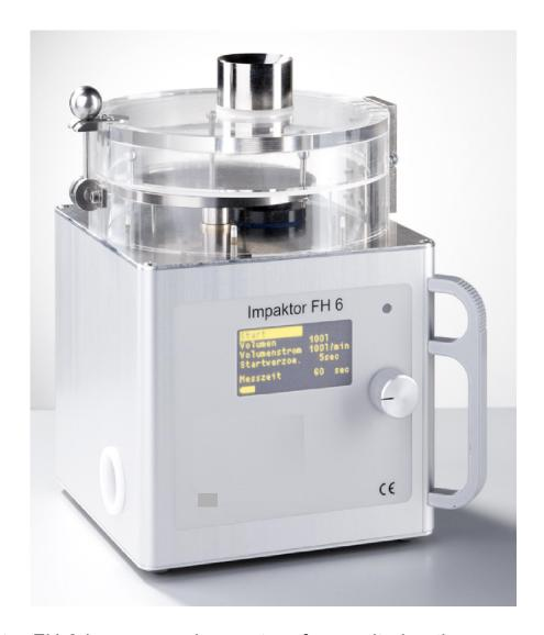
The Impaktor FH-6 is a measuring system for monitoring the germ content in the air. The system is applicable for the impaction method as well as for the filtration method.
